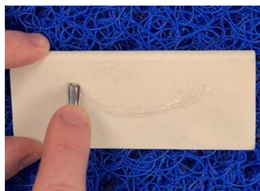
Take the back side of the instrument, the convex surface and place onto the stone. Raise the angle of the instrument up to approximately 45 degrees, so the back of the tip of the blade touches the surface of the stone.
