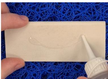
Drip a small amount of oil (MD30) onto the flat surface of your stone in the shape of a smile or a shallow "U" shape.
