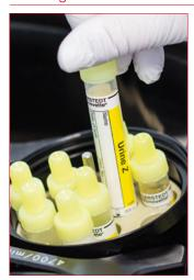
Used directly as a centrifuge tube, the Urine Monovette® reduces analysis time. Once the supernatant has been decanted, the plunger can be pushed back up and the sediment hygienically removed.
