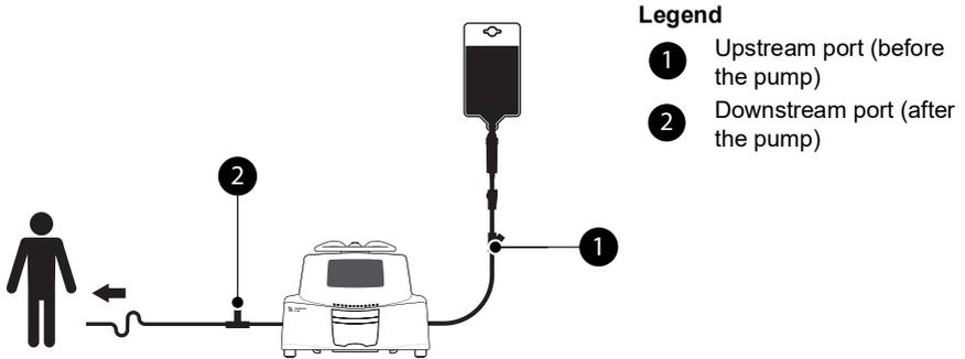
**Figure 13.1:** Needle-Free Ports
