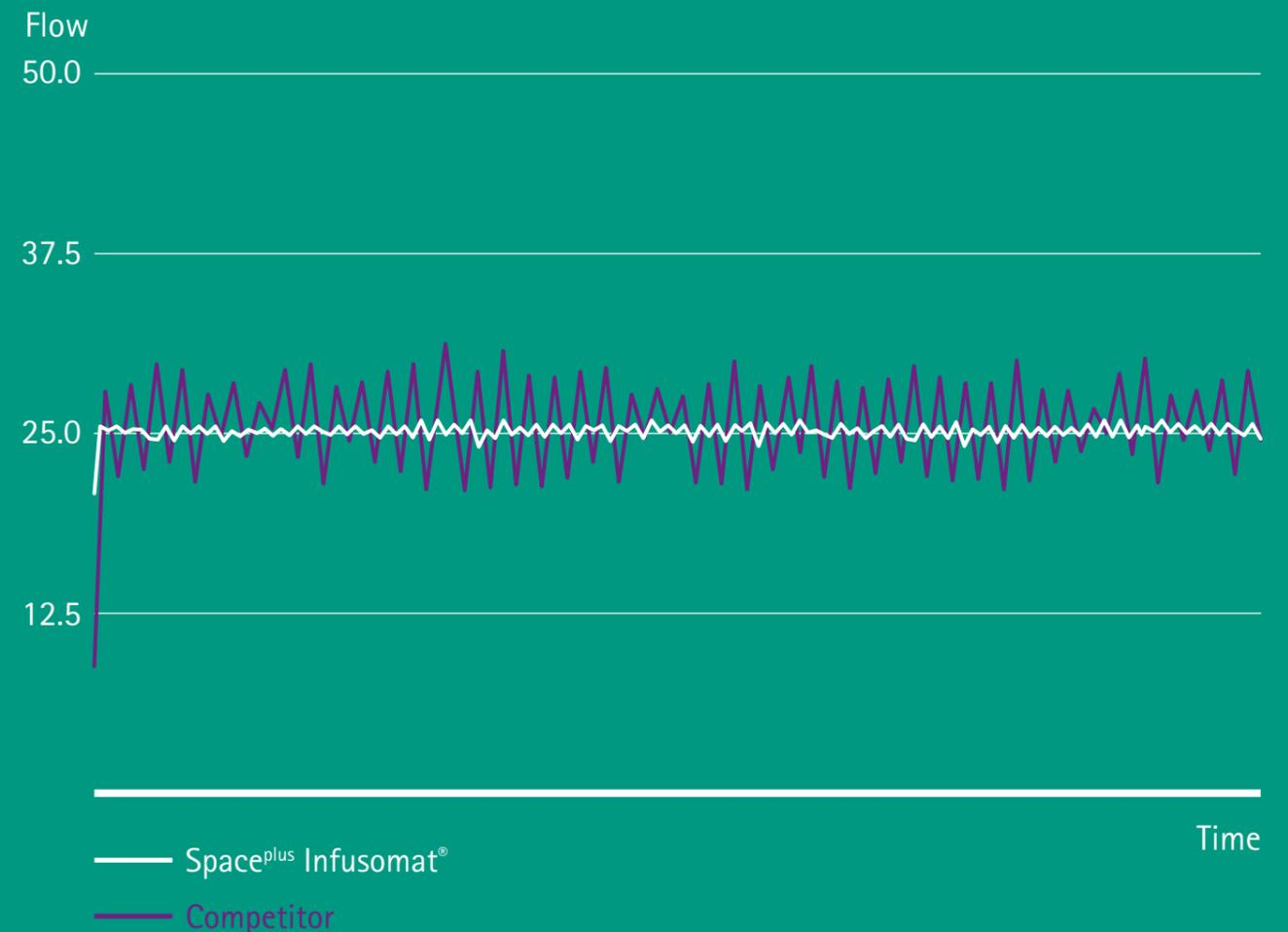
These graphs show the accuracy and uniformity of flow over time. It must be remembered that the delivery characteristics and the delivery accuracy are significantly affected by the disposable used.
